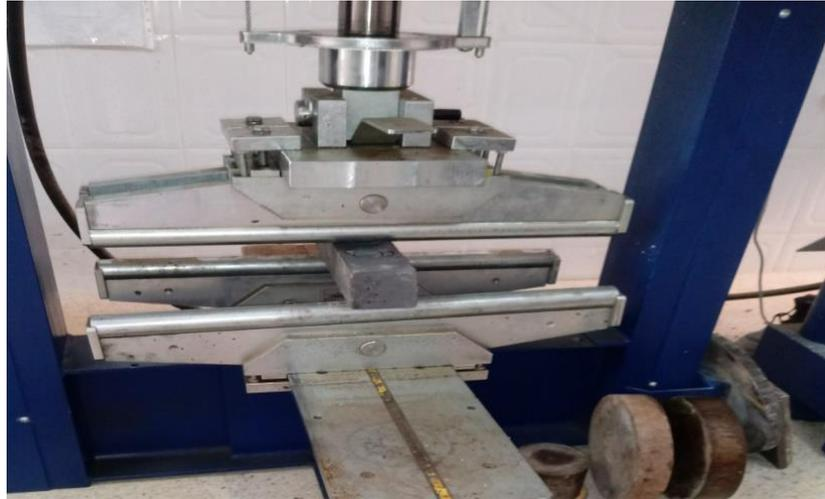
Figures (I.15) Bending tensile tests.
