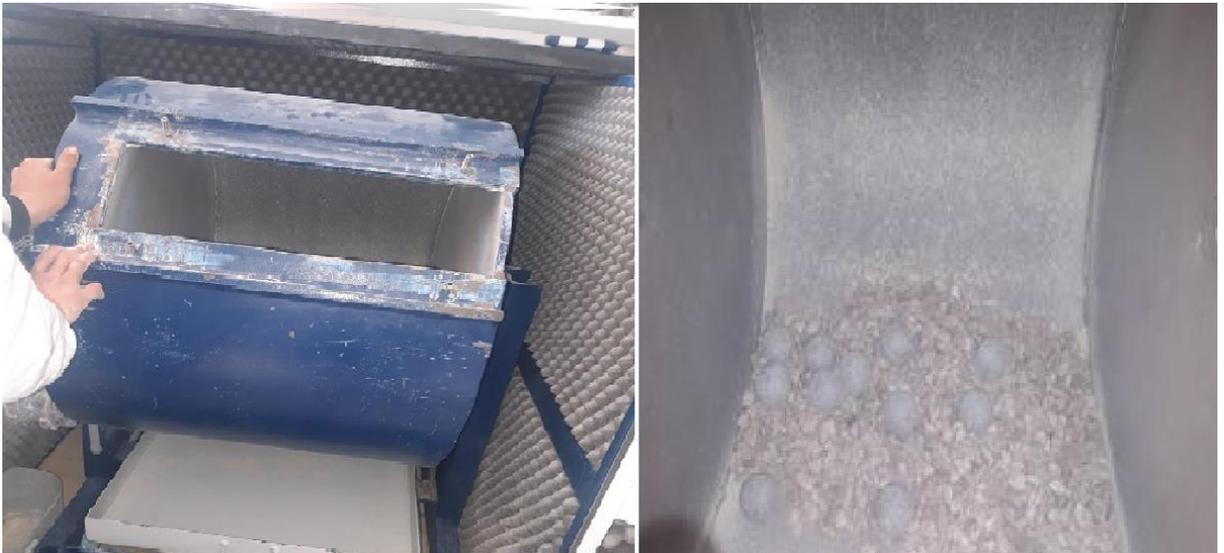
Figure (III.5) Los Angeles abrasion test
