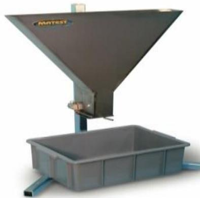
Figure (I.11) Equipment for V-Funnel test.
