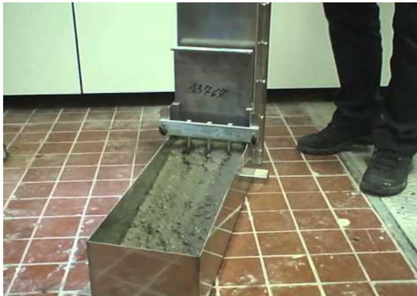
Figure (I.9) Procedure of L box test.
