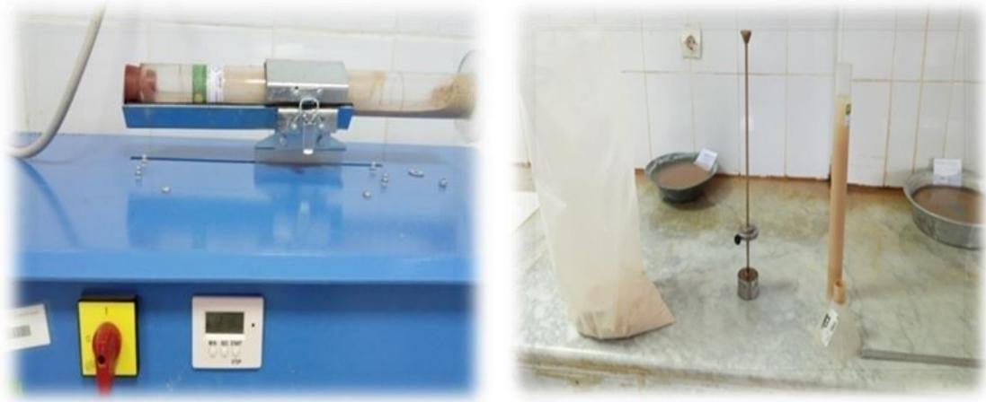
Figure(III.3) The sand equivalent test.
