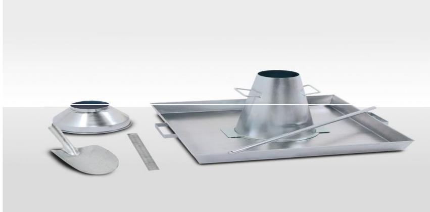
Figure (I.3) Equipment for slump flow test.
