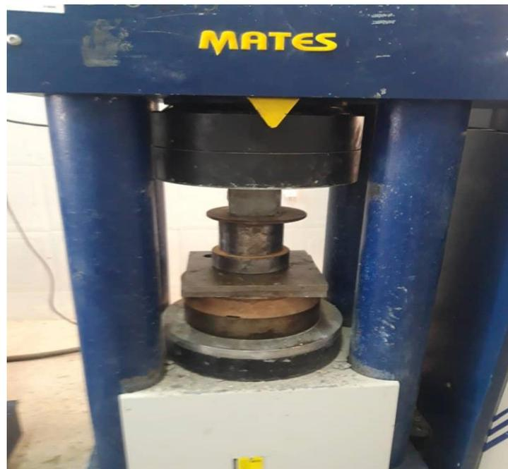
Figure (IV.1.) compressive strength machine.
