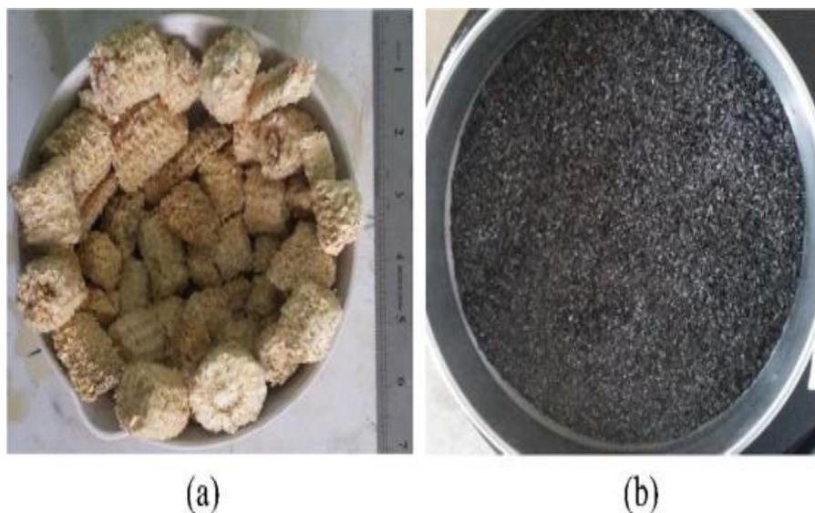
Figure (II.5) Stages access to corn cob ash.
