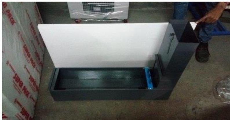
Figure (I.7) Equipment for L box test.
