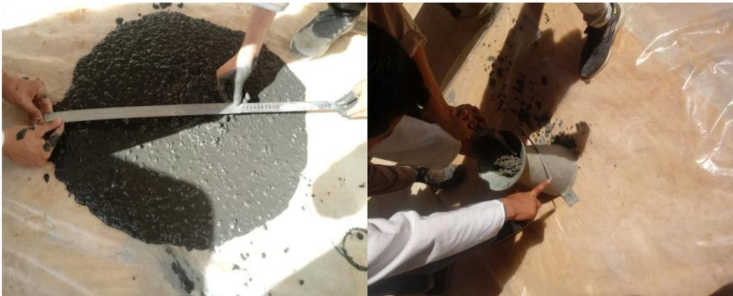
Figure III.8 Slump Flow Test
