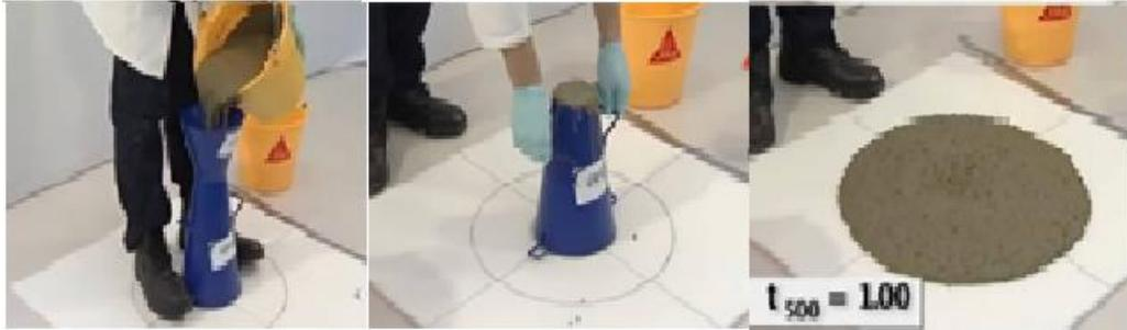
Figure (I.5) Procedure of slump flow test.
