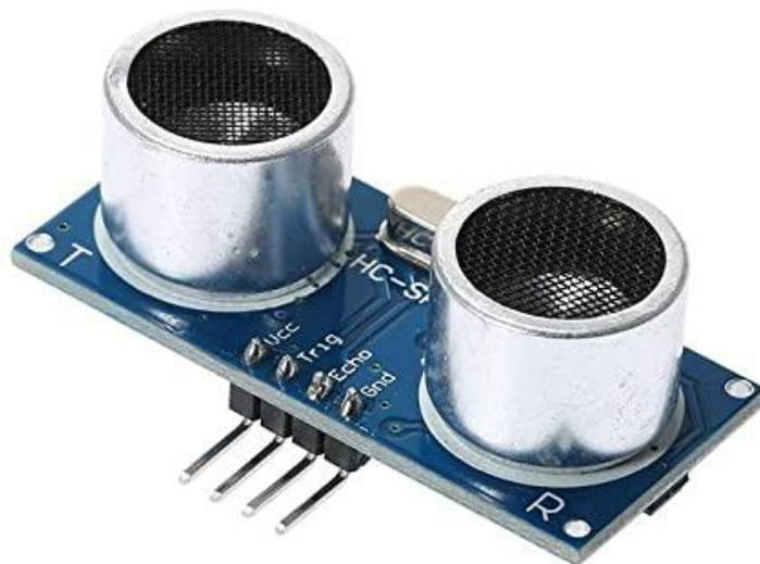
Figure 21 : capture ultrason
