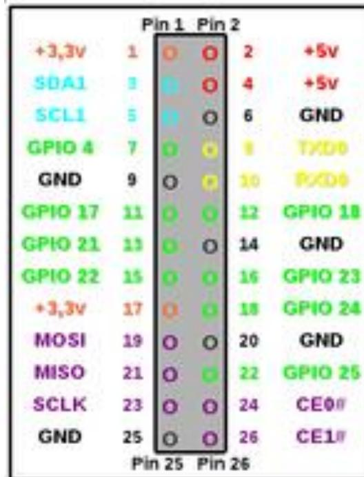
Figure 2.5:Raspberry B 512 Mo - GPIO 26 pins
