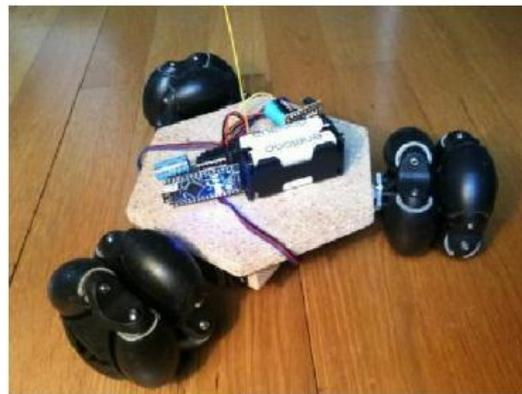
**Figure 1.8: Robot mobile omnidirectionnel.**
