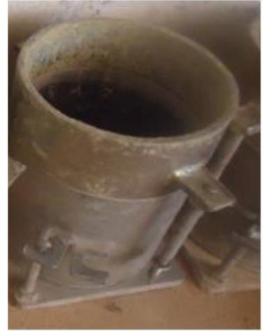
*Photo I-5-Moule de Proctor normal*
