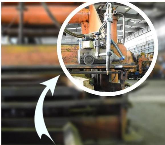
FIGURE 8 : UNE PHOTO PRISE DE DISPOSITIF D'OXYCOUPAGE.
