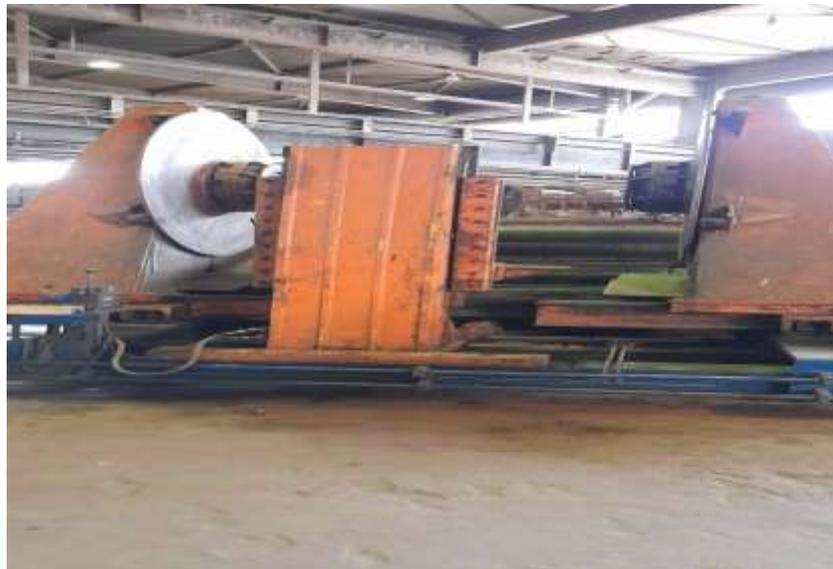
**Figure III.2. supporte bobine**
