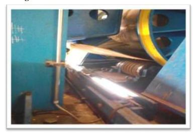
Figure I-3: Dispositif de debobinage.
