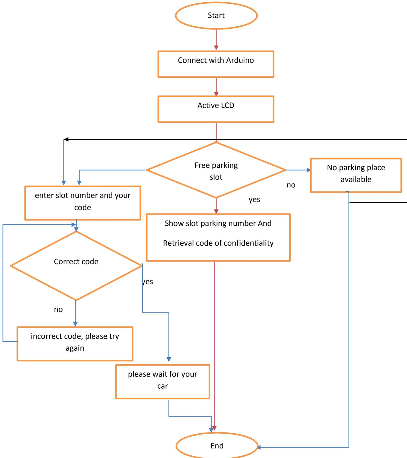
Figure II.2: Flowchart of display procedure.
