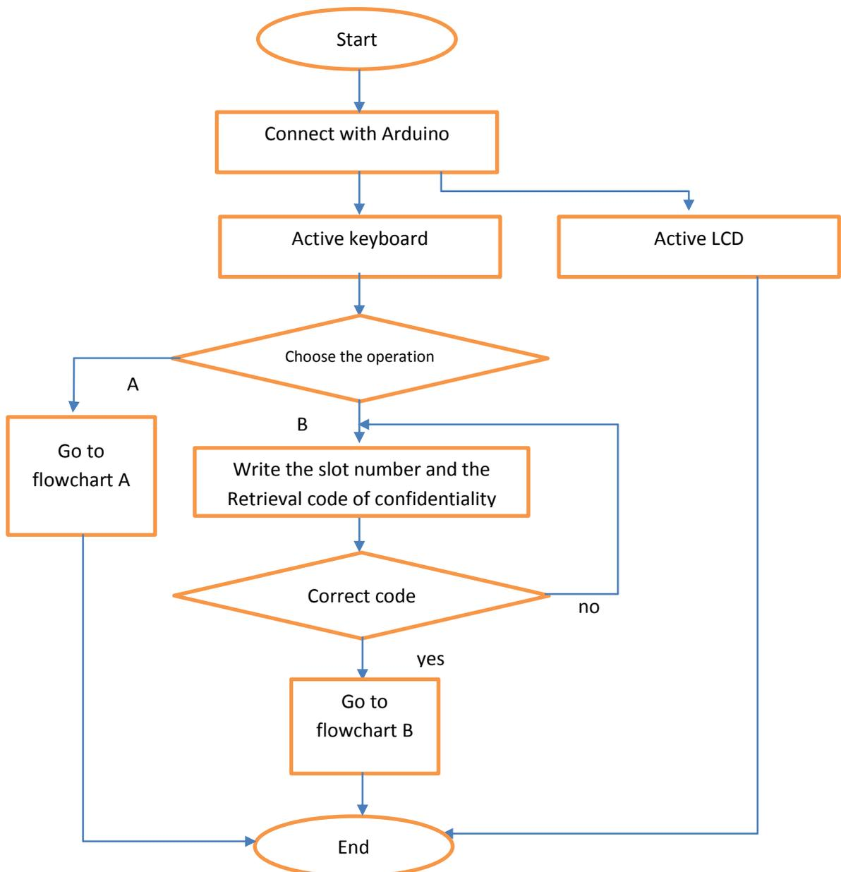
**Figure II.5:** Flowchart of keyboard using procedure.
