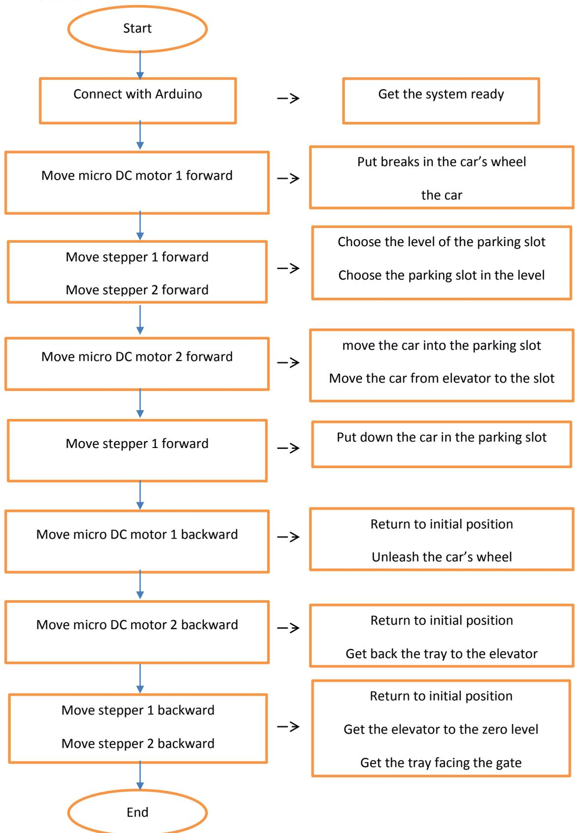
Figure II.6: Flowchart A of parking in procedure.
