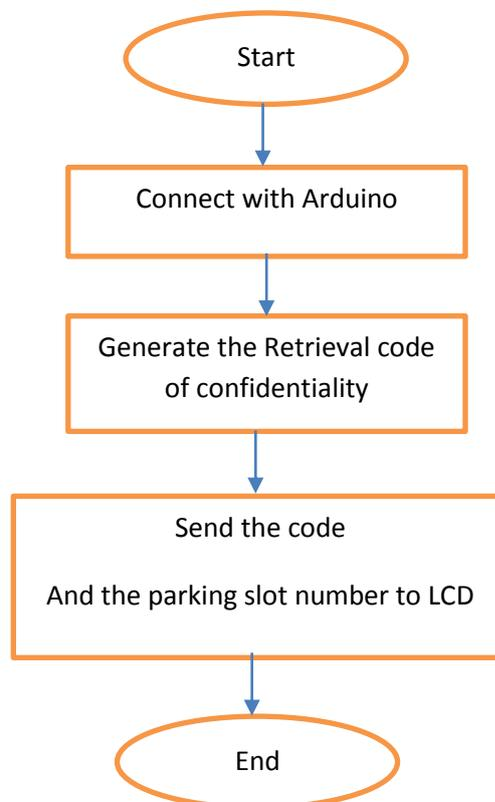
**Figure II.4:** Flowchart of generating/regenerating the code procedure.
