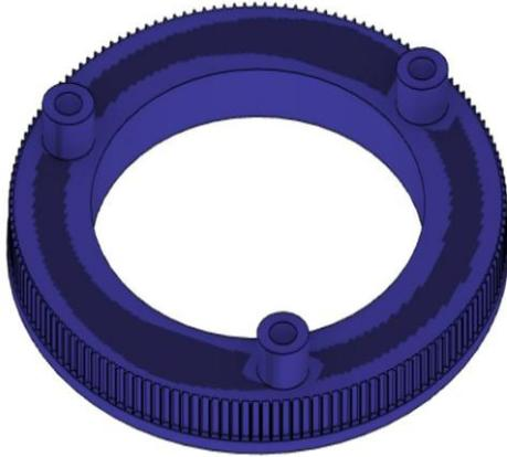
**Figure III.2:** the design of stirring gear.
