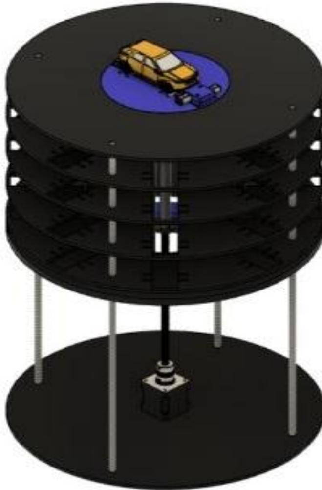
**Figure III.1:** the design the prototype with the software Fusion 360.
