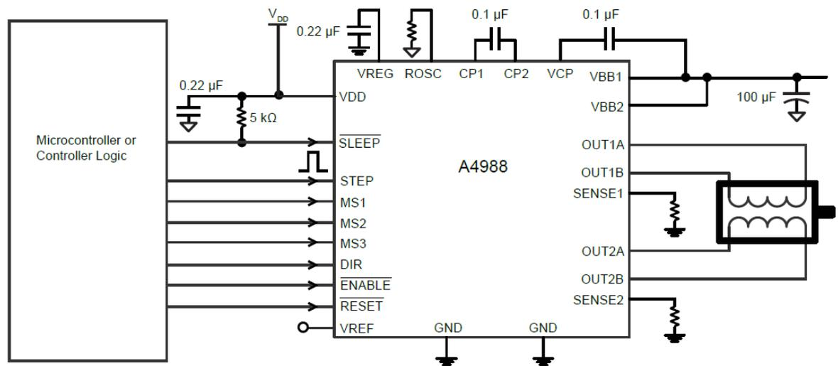
**Figure II.8:** Typical Application Diagram [35].
