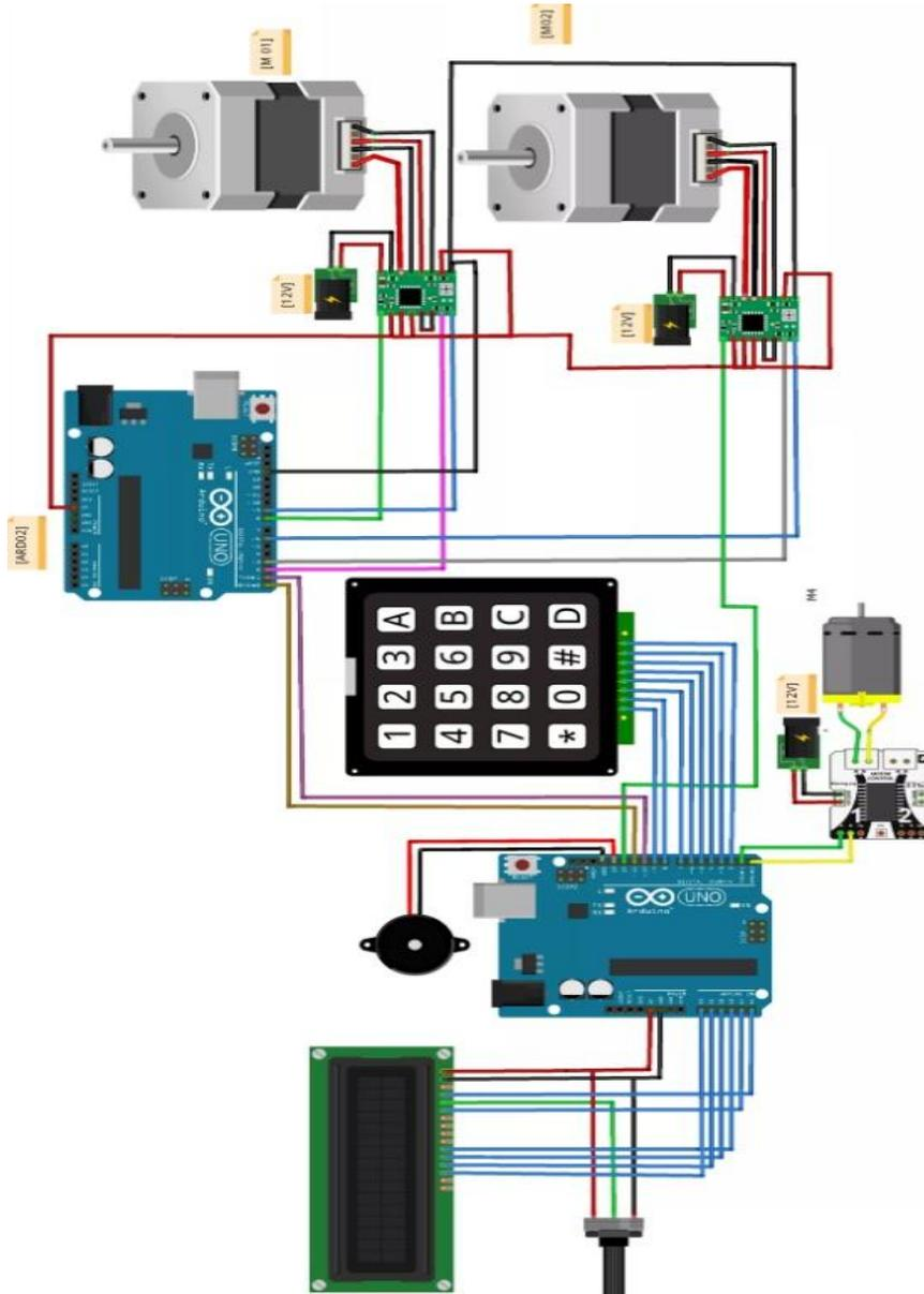
**figure III.7:** the electronic circuit designed using Fritzing.
