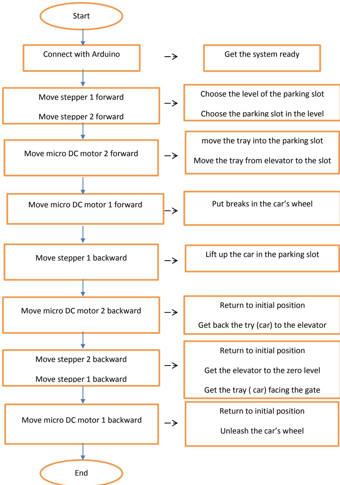
**Figure II.7:** Flowchart B of parking out procedure.
