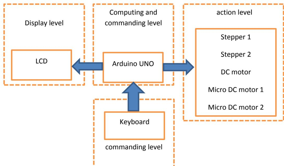
**Figure II.1:** Block Diagram of the system.
