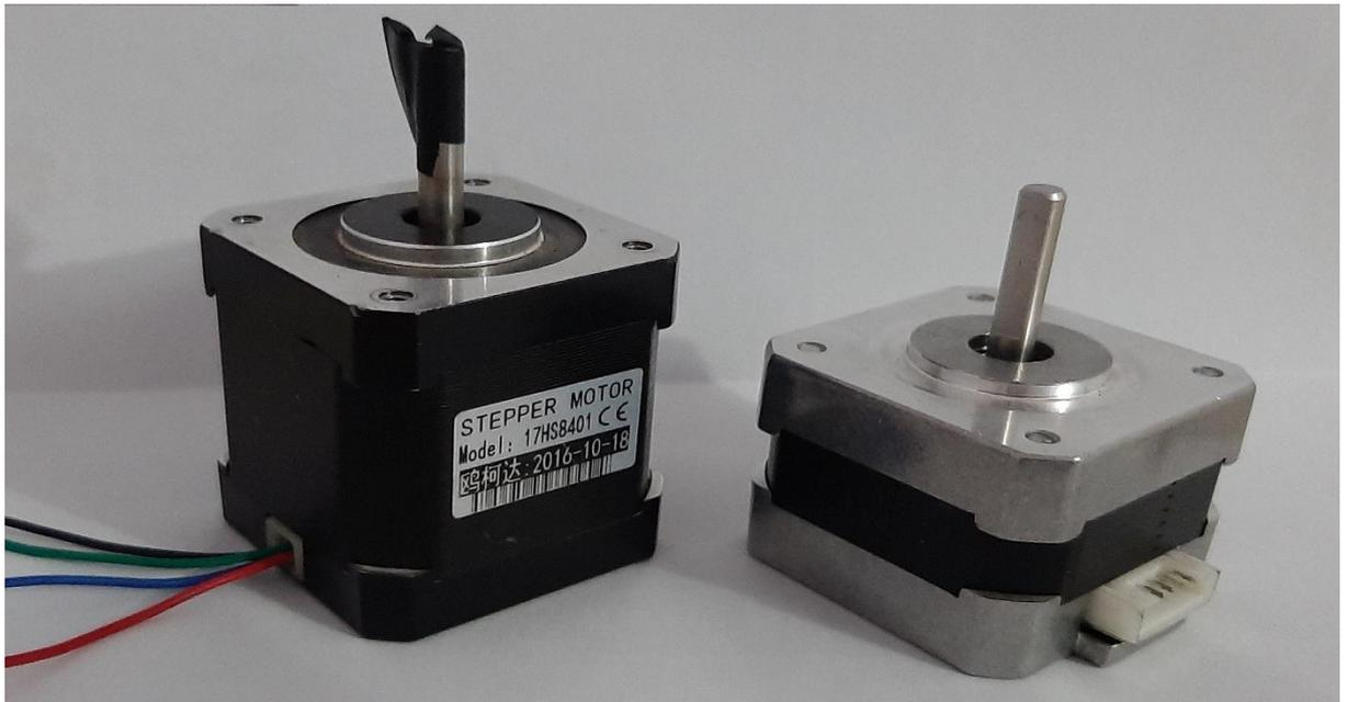
**Picture II.10:** stepper motor 17HS8401 and stepper motor 42SHD0001-24B.
