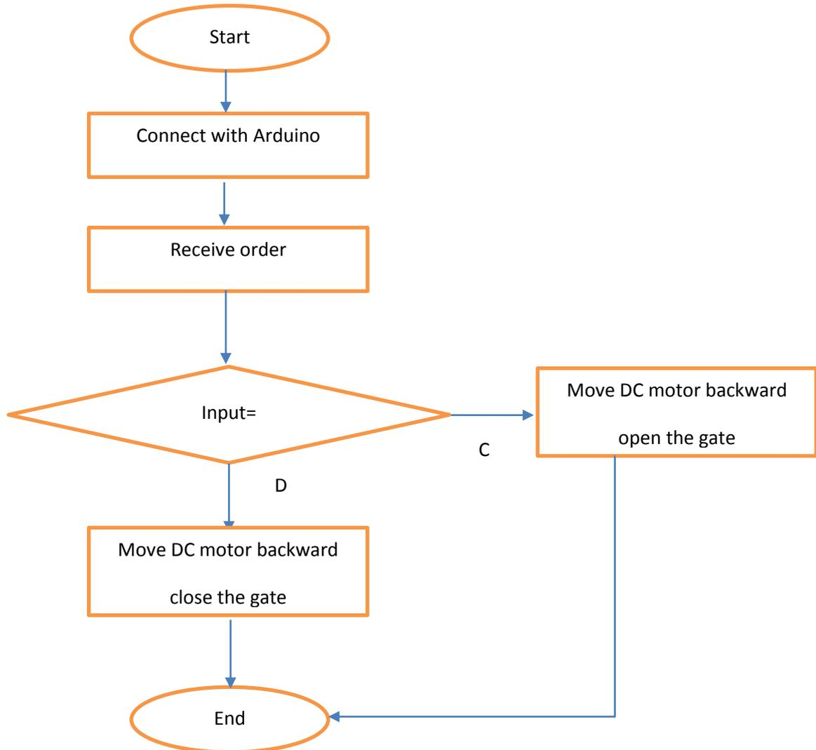
**Figure II.3:** Flowchart of opening/closing the gate procedure.
