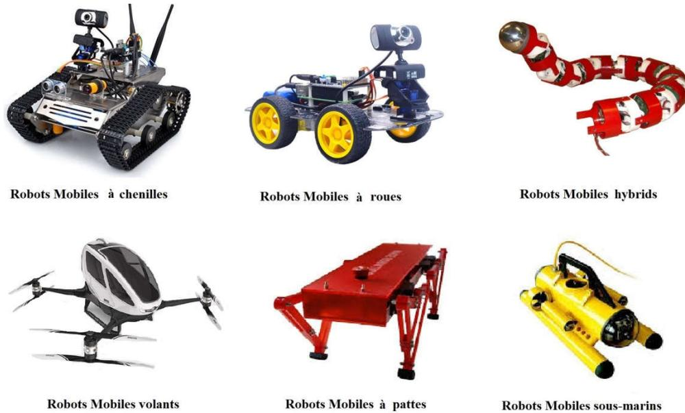
**Figure I.2:** La classification des robots mobiles.
