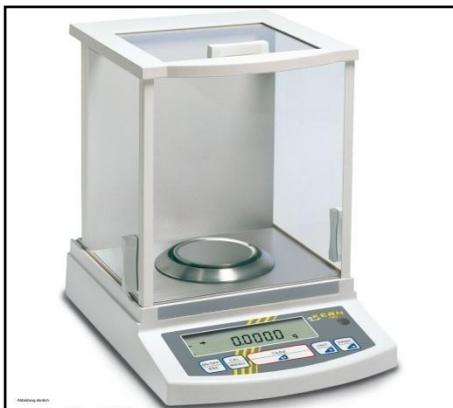
**Figure III.13.** Balance KERN ABJ10mg-220g [155]
