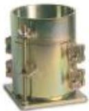
**Fig.II- 10.**—Moule Proctor normal.
