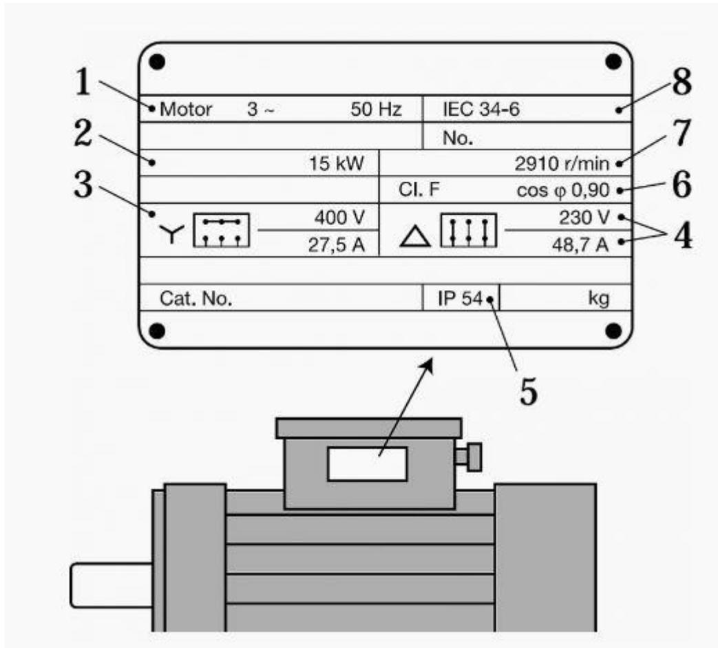
**Figure I-5:** Example nameplate of induction motor
