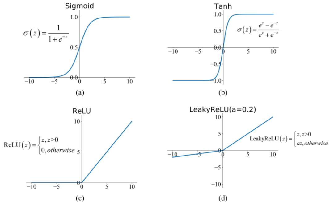
**Figure III-3 :** Commonly used Activation Functions.
