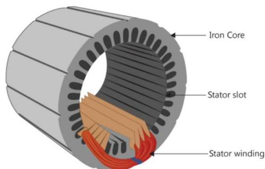
**Figure I-2:** The stator of induction motor
