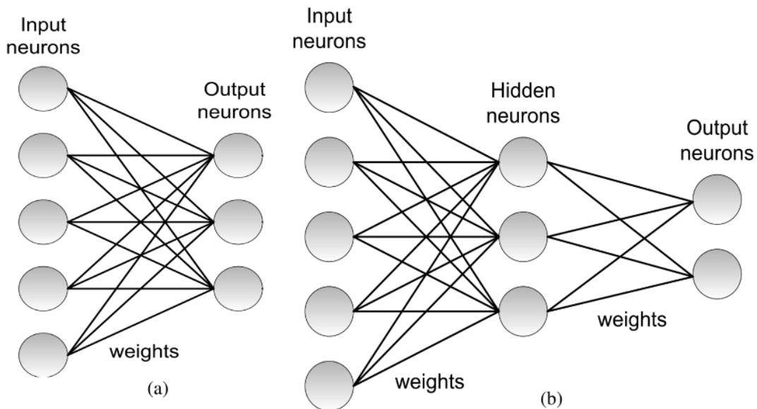
**Figure III-4:** Different Models of Neural Networks.
