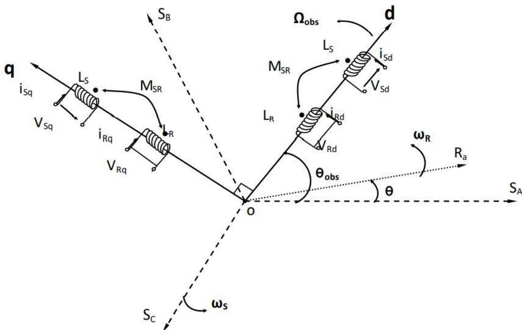
**Figure II-2:** Rotating frame of axes ( d– q)
