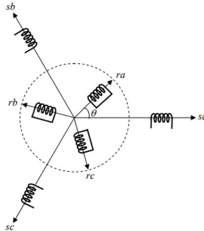
**Figure II-1:** Schematic representation of a three-phase induction machine.
