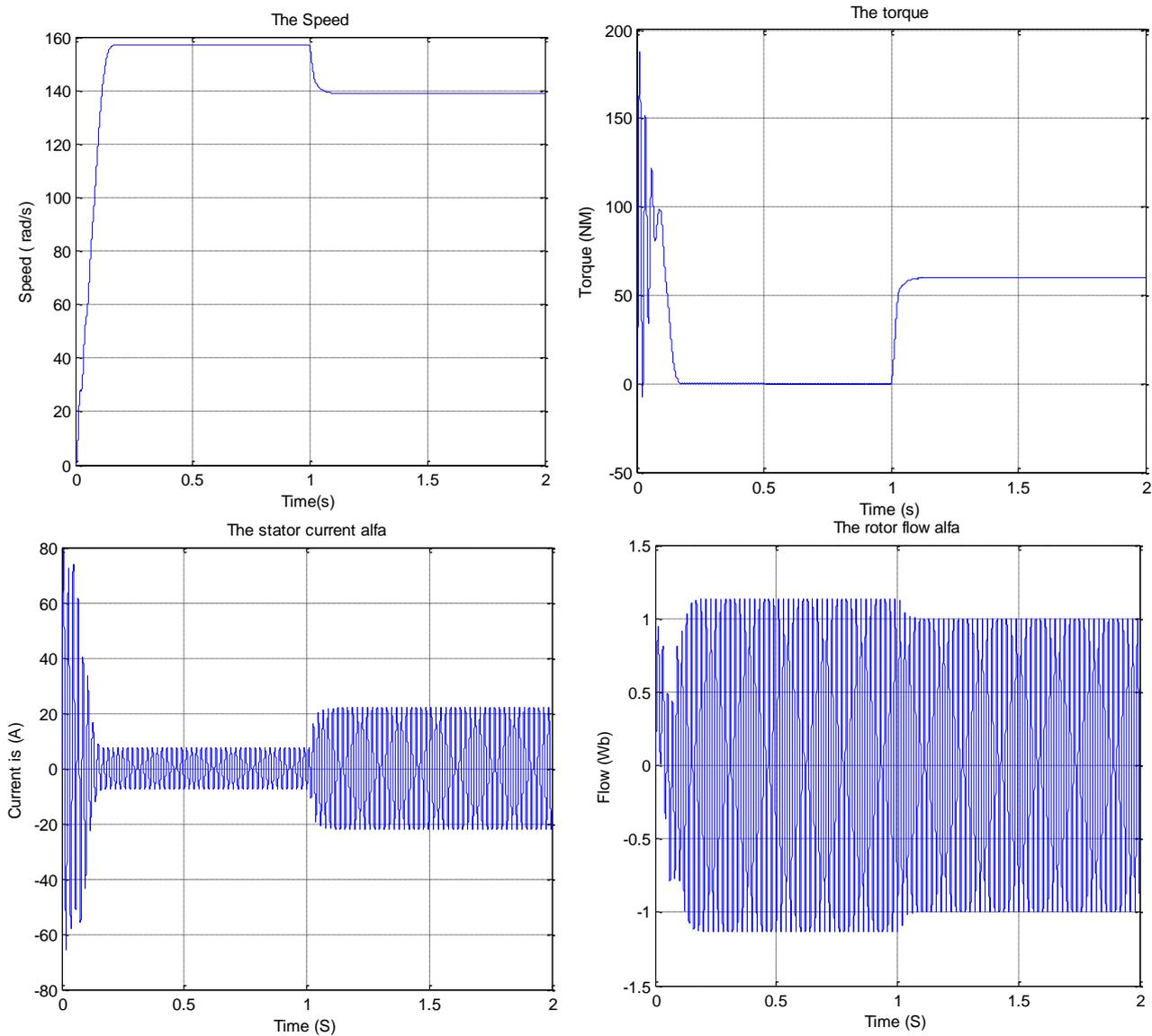
**Figure IV-3:** Simulation results of the induction machine model under load
