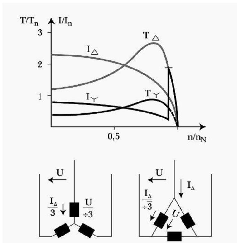
**Figure I-6:** motor torque and current in star and delta connections
