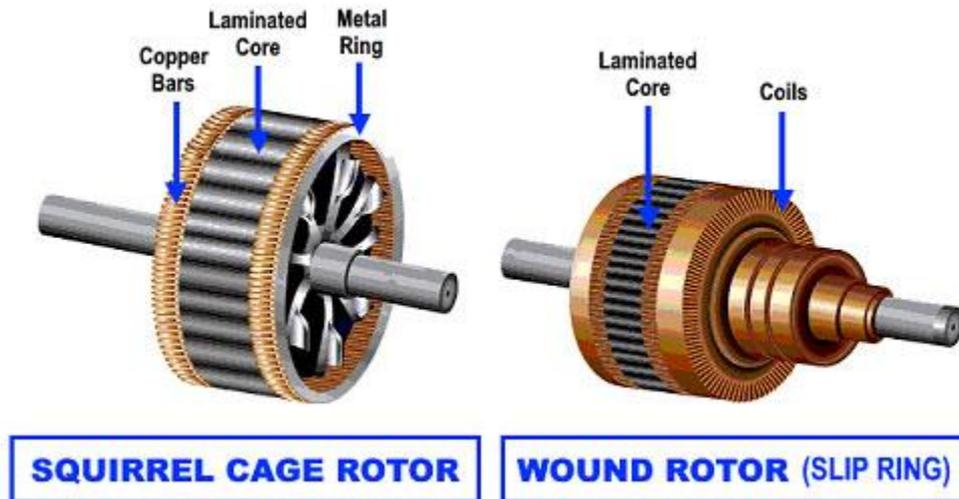
**Figure I-3:** The rotor of induction motor
