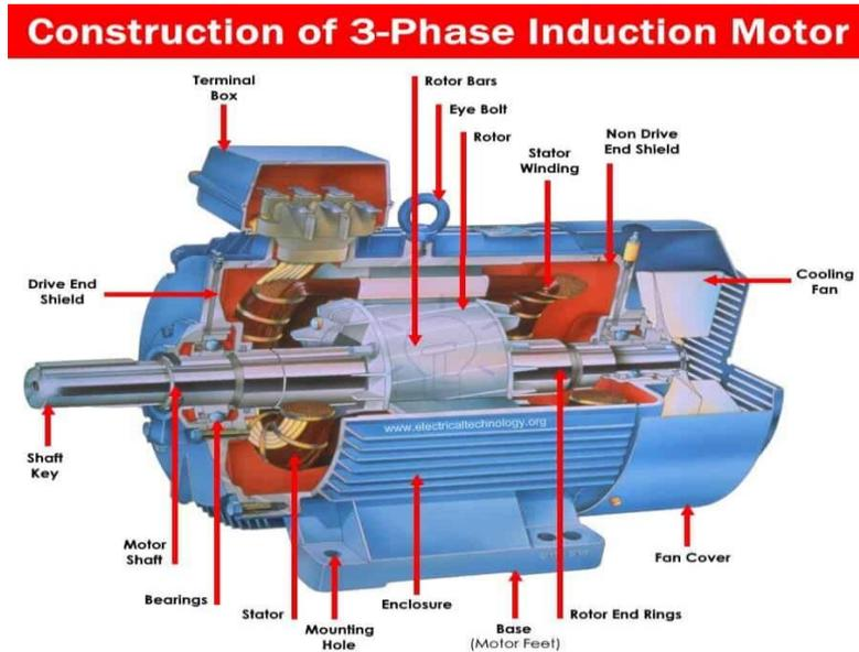
**Figure I-1:** construction of 3-phase induction motor
