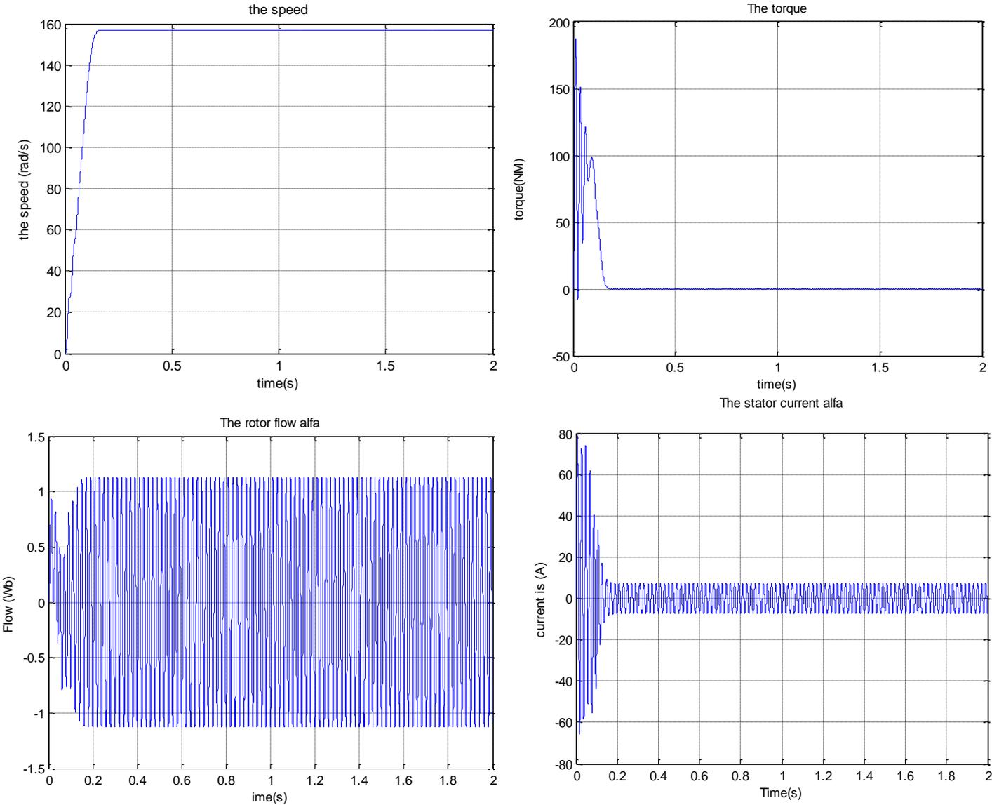
Figure IV-2: Simulation results of the induction machine model during no load start
