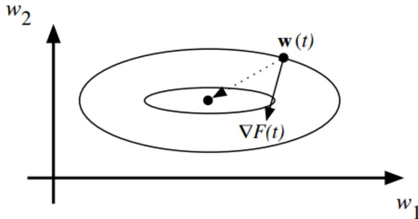
**Figure III-8:** Gradient descent trajectory.
