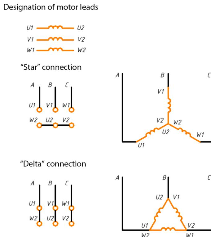
**Figure I-4:** coupling of induction motors (star and delta)
