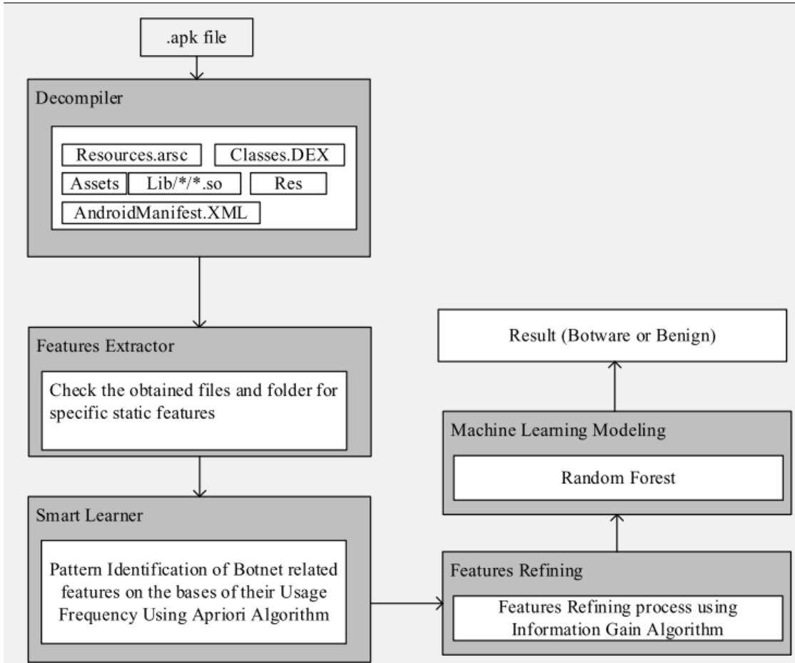
Figure 3.5: Anwar et al. [50] method diagram
