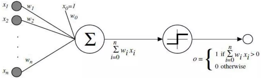
Figure 4.1: A diagram showing how the Perceptron works [77]
