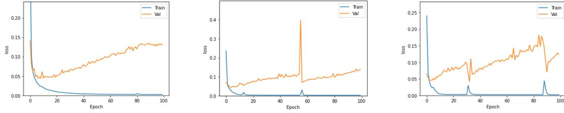
: (a) MLP with 1 hidden layer model loss by epochs : (b) MLP with 2 hidden layers model loss by epochs : (c) MLP with 3 hidden layers model loss by epochs
