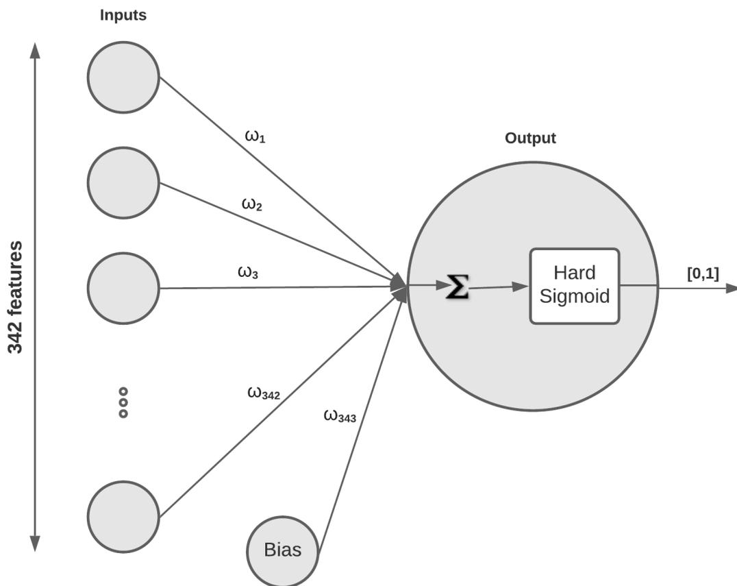
Figure 4.2: Proposed method using the Perceptron model diagram
